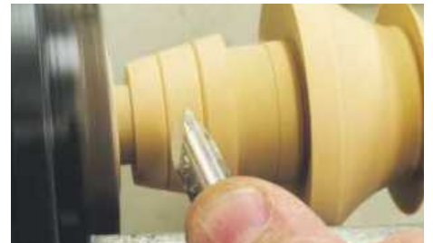
▲ Pic.6 Make the tree container look like half a barrel. A simple taper with some grooves cut in it gives a good and easily achievable effect
